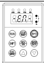
Fig.a electrification, display-EN-
